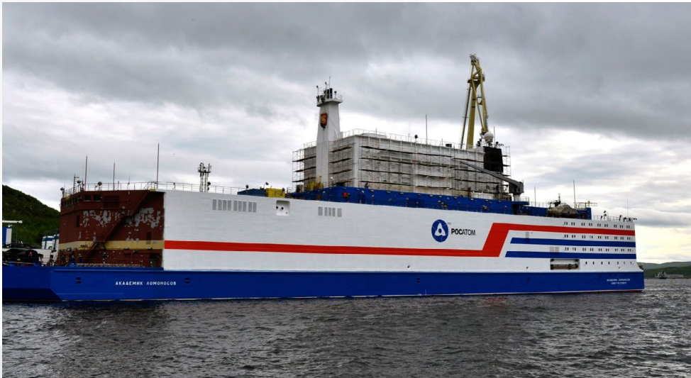
Two small reactors on the first purpose-built floating nuclear power plant, harbored at the town of Pevek in northeast Russia, started supplying electricity
